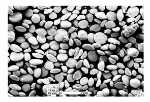
The electron microscope photo shows the uniform round shape of the starch based spray powder. The amount of fine particles is very low.
