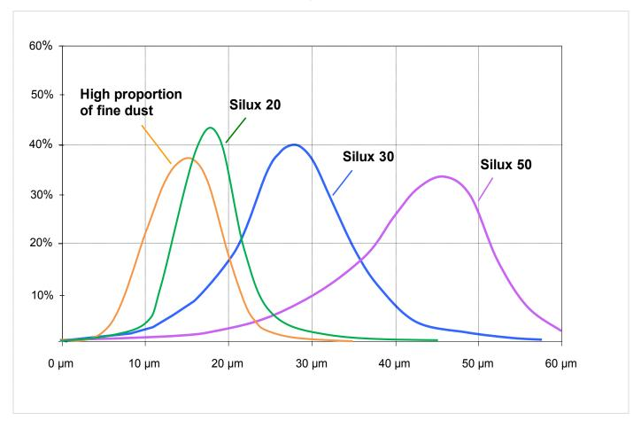
BöttcherPro Silux Spray Powders are fine dust reduced and have only a small amount of particles below 10 microns.
