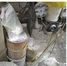
1-kg plastic pouches with screw cap are much better to handle. No spillage of spray powder when refilling
